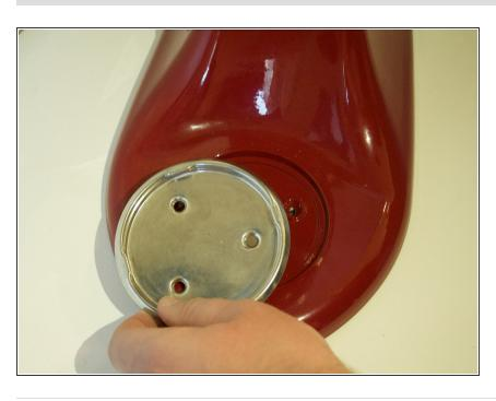
Remove the bowl screw cap by grabbing the side and lifting up on it.
