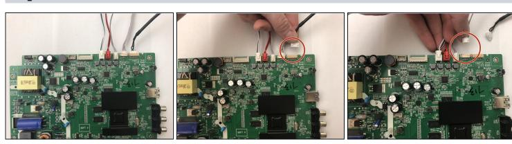
• There are 5 wires attached to the motherboard. Remove the two thicker white wires to the right of the red wire.
