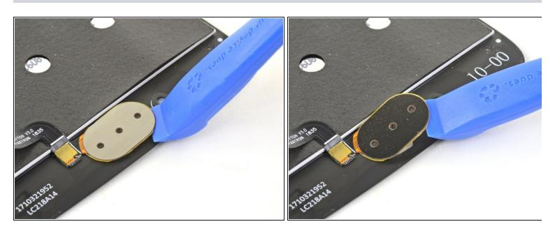
• Use an opening tool to pry up and loosen the fingerprint sensor from the screen.
