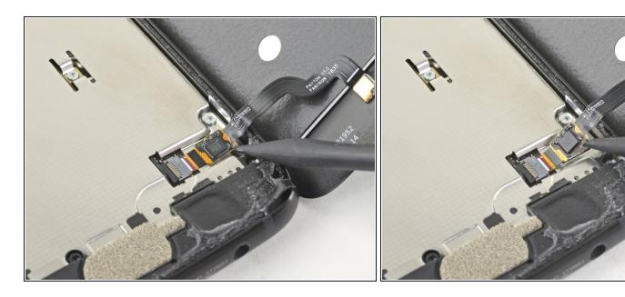
Slide the point of a spudger underneath the fingerprint sensor cable and gently pry up to loosen the cable from the phone.
