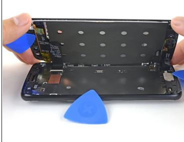
⚠ Do not try to remove the screen yet—it is still attached to the phone by delicate flex cables.
