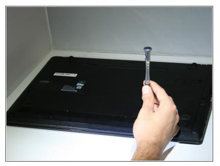
Unscrew the two screws using a Phillips #0 screwdriver.
