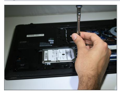
• Unscrew the four screws around the Hard Drive using a Phillips #0 screwdriver.
