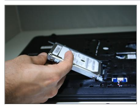
• Slide the hard drive over and remove it from the device.
