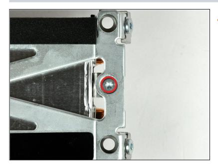
Remove the 4.3 mm T10 Torx screw securing the heat sink to the heat sink bracket.
