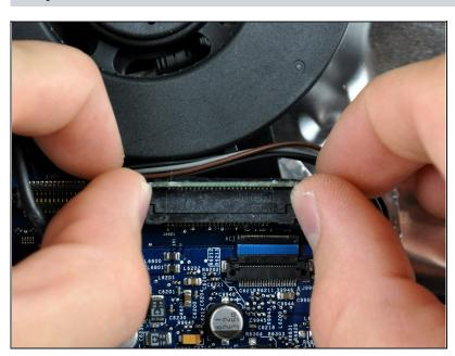
Push the optical drive cable connector toward the top of your iMac to disconnect it from the logic board.
