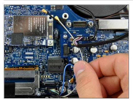
Move both AirPort antennas toward the lower edge of your iMac, out of the way of the logic board.
