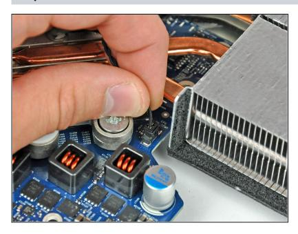
Disconnect the heat sink temperature sensor connector by pulling it straight up from its socket on the logic board.
