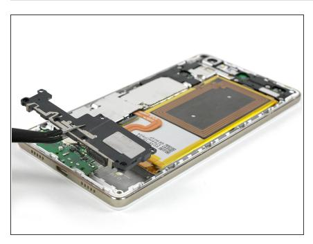
Remove the loudspeaker carefully.
