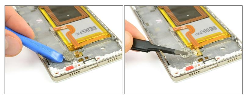
Pry off the vibrator using a plastic opening tool.
