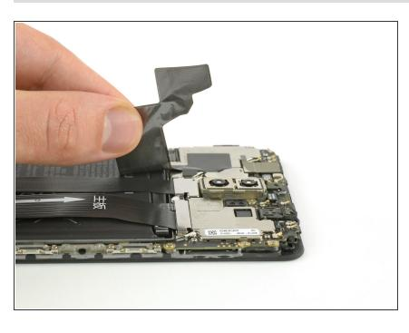
Carefully peel off the plastic sticker that holds both cables to the battery.
