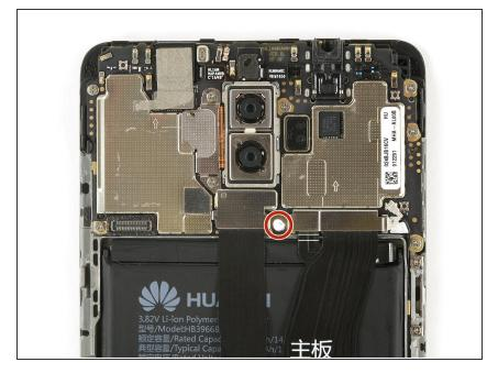
Remove the water indicator sticker and the Phillips #00 screw beneath it, that holds the cable bracket in its place.
