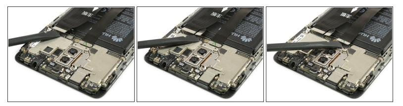
• Use a spudger to disconnect the interconnect, the battery and the display flex cable.
