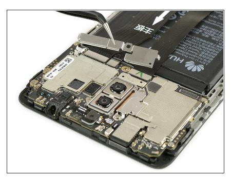
Remove the cable bracket.
