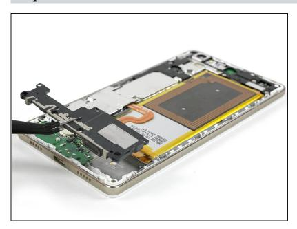
Remove the loudspeaker carefully.
