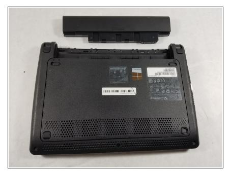
While keeping both of the tabs in the unlocked position, grab the battery and pull outwards, until the battery slides out from the rest of the computer.
