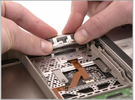
Insert the new latch by rotating the clip up and pushing the latch into place. Then rotate the clip back down, pushing in at the area where the clip bends around the latch. Make sure to insert the clip fingers back into their slots.
