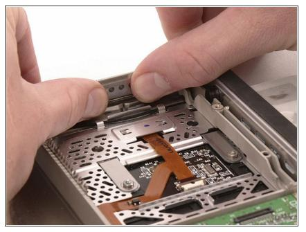
• Use your thumbnails to push in and then lift the two fingers of the latch clip over the restraining bar.
