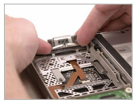
Now use your index fingers' nails to pull at the "elbows" of the clip, rotating it upward approximately 90 degrees, or until the latch pops out
