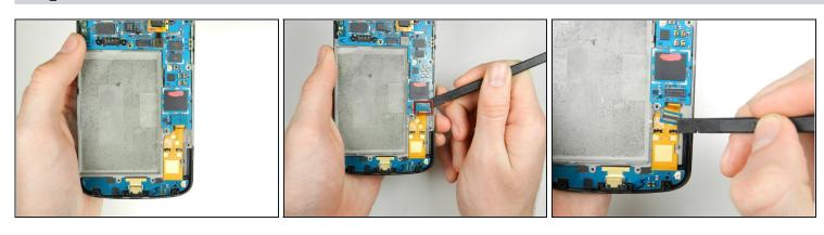
Remove the tab located in the bottom right-hand corner of the motherboard attaching the motherboard to the front display assembly using a spudger.
