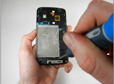
• Remove the two 4.8 mm screws that hold the speaker enclosure together using the Phillips 00 screwdriver.
