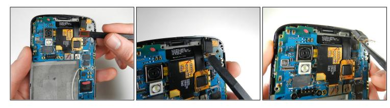
• Using a spudger, pop off the gray connector on the top right of the motherboard.
