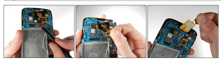
• Gently pry the metal tab up using a spudger, and lift up the disconnected black flap.
