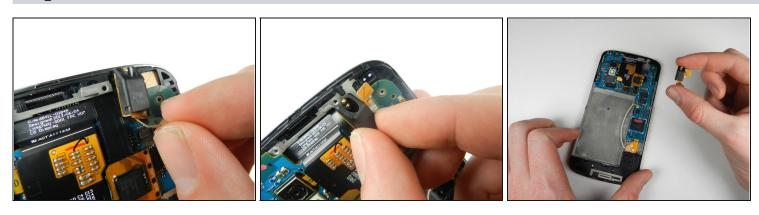
• Gently lift the audio jack upwards and to the left to remove it from the motherboard.
