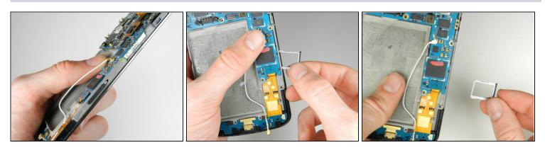
• Remove the Sim Card and the Sim Card metal tray.
