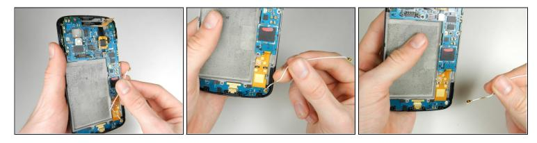
• Remove the white antenna interconnect cable that attaches the motherboard to the bottom right-hand corner of phone by pulling on it gently.
