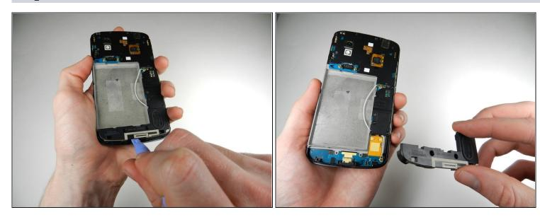
• Gently pry the speaker up and away from the back of the phone using a plastic opening tool, and lift it out of the phone.
