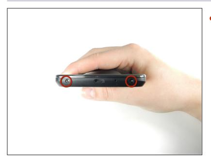
Remove the two screws from the bottom of the phone with a T5 Torx Screwdriver.
