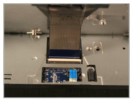
lift up bottom of keyboard slightly, to access keyboard ribbon
