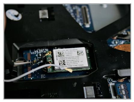
• Remove wifi wires by lifting up
