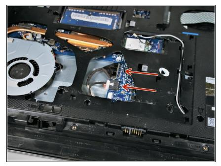
• locate power and monitor cable on bottom side next to fan
