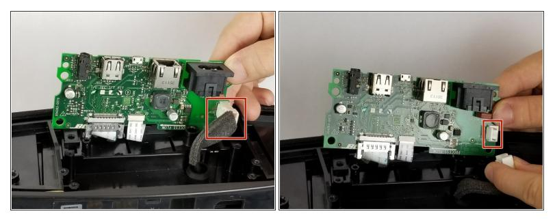
• Remove the white cable by pressing on the side of the connector with a tab and pulling backwards.
