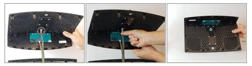
• After lifting the cover, you will see two ribbons attaching the cover to the speaker. Gently remove these ribbons by pulling straight down.
