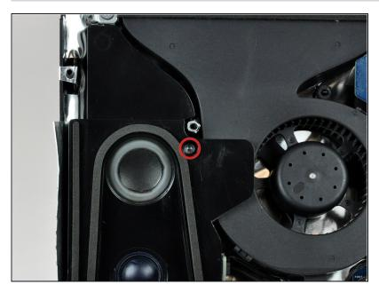
Remove the single 28 mm T10 Torx screw securing the left speaker to the rear case.
