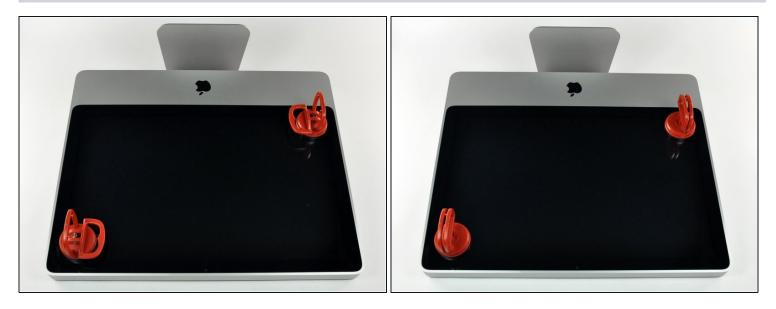
(i) The glass panel is fixed onto the front bezel with fourteen magnets around its perimeter.
