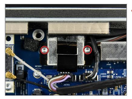
Remove the two 5.3 mm T6 Torx screws securing the data display cable to the logic board.
