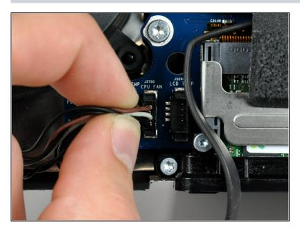
Disconnect the CPU fan connector from the logic board by pulling it straight up from its socket.
