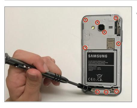
Remove all 11 screws by using the J000 phillips head from the 64 Bit Driver Kit.
