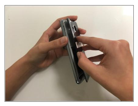
Separate the back casing from the phone by carefully using your fingers to pry it apart.
