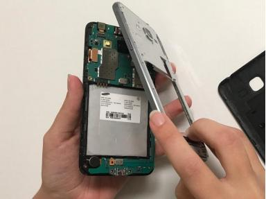
• Use the flat side of the metal spudger to remove the middle frame bezel, and replace.
