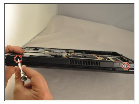
Using the PH1 screwdriver remove the two .75 mm screws from the hinge side of the laptop.
