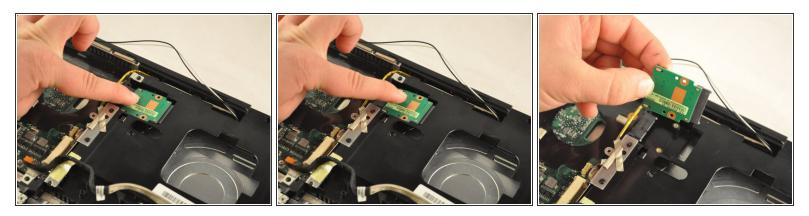
• Slide and lift the RAMdrive out of its port.
