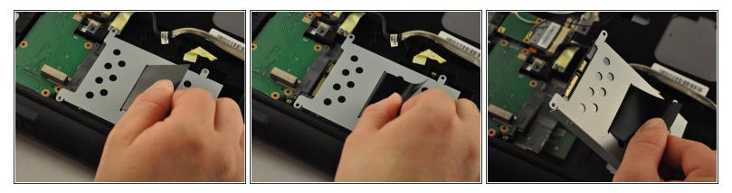
• Pull on the black tab on the driver to slide the driver back, and lift the driver out of the laptop.
