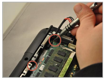
• Using the PH1 screwdriver, unscrew the two .75 mm screws from the top-left corner of the motherboard.
