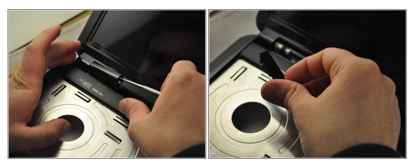
• Use the metal spudger or opening tool to pop out the plastic hinge covers.
