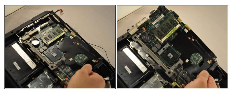
There is a ribbon cable connected to the back of the motherboard. Be careful not to break the ribbon cable.
