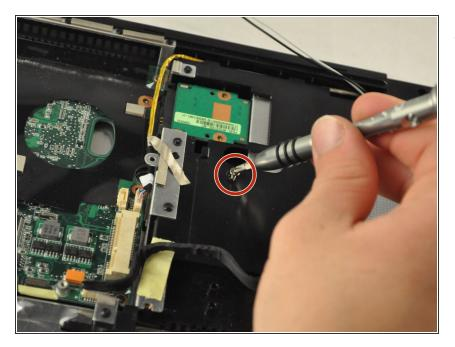
Using the PH1mm screwdriver, remove one .5 mm screw from the disk drive, located inthe top-right corner of the laptop.
