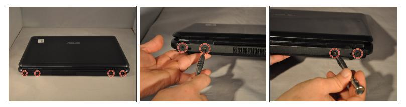
• Using the PH1 screwdriver, remove the four 4.75 mm screws that are located on the vent panel.
