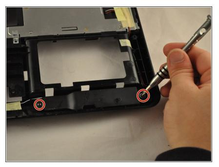
Using the PH1 screwdriver, remove the two .75 mm screws out of the speaker, located in the bottom right corner of the laptop.
