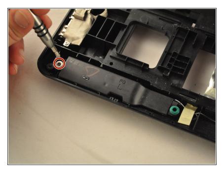
Using the PH1 screwdriver, remove the one .75 mm screw from the other speaker located in the bottom left corner of the laptop.
